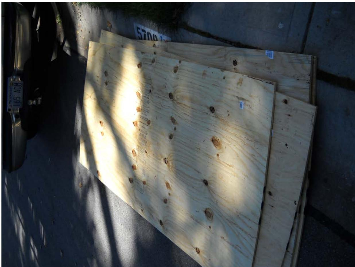
Photo #1 With CDX plywood, we can see wood grain.
