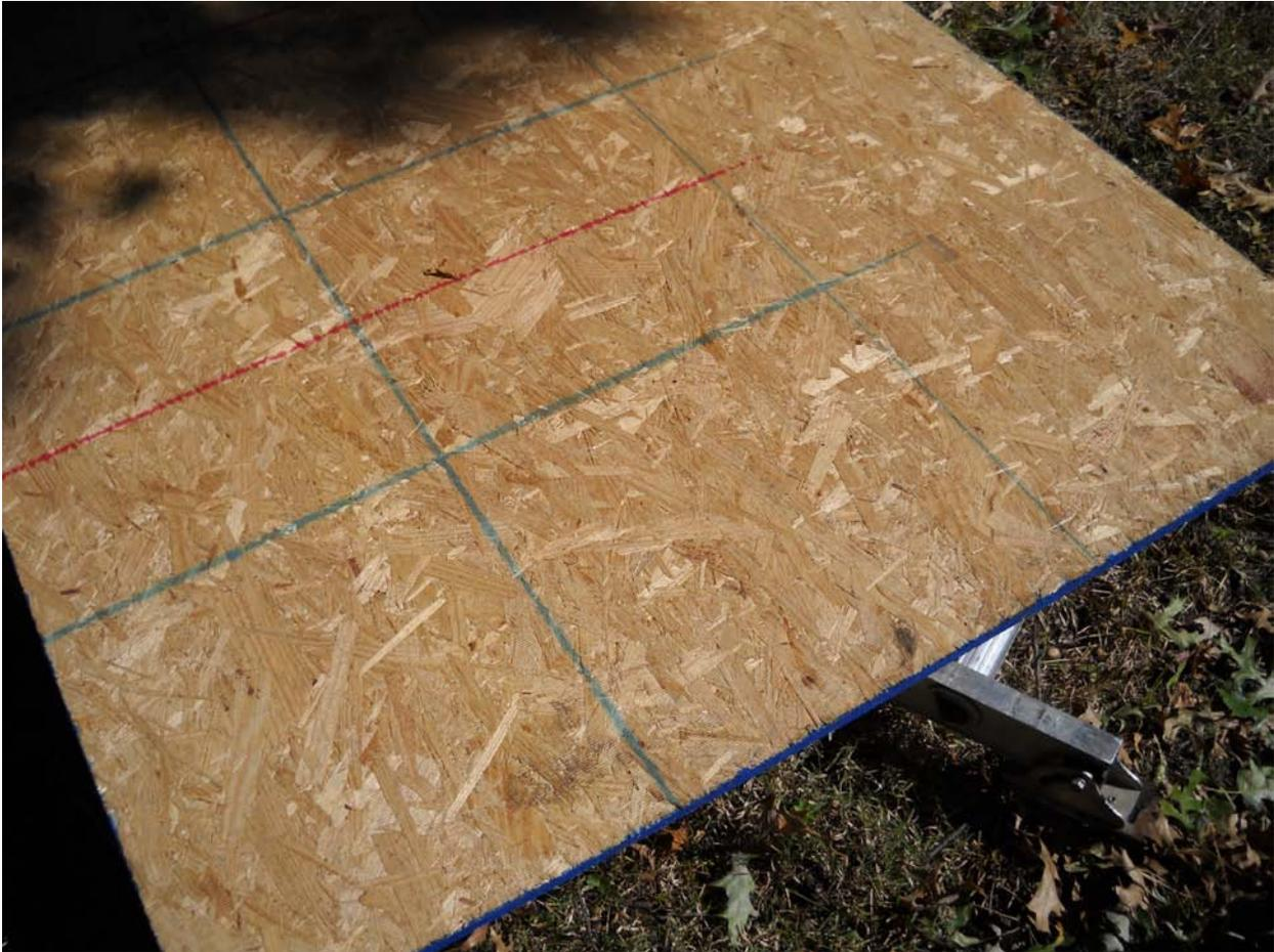
Photo #3 OSB has a very different look than CDX plywood.
